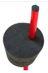
Push the hose through the thin topmost layer. The punch residue remains attached to the hose ends.
