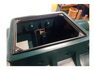
Check that the bottom riser has been trimmed and confirm the 5mm pilot holes have been drilled out. If not, use a 5mm drill bit and use the drill spots on the bottom of the tool (3 on each of the long side and 2 on each of the ends)
