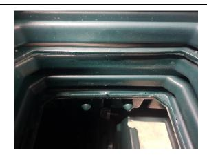
Take the lid frame and, if necessary, refix the neoprene strip to the inside surface, as close to the edge as possible.
