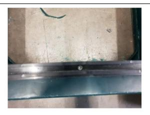
Reattach the lid using the original countersunk set screws
