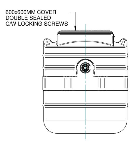
Available in single or twin pump configurations for rain water, effluent or sewage
